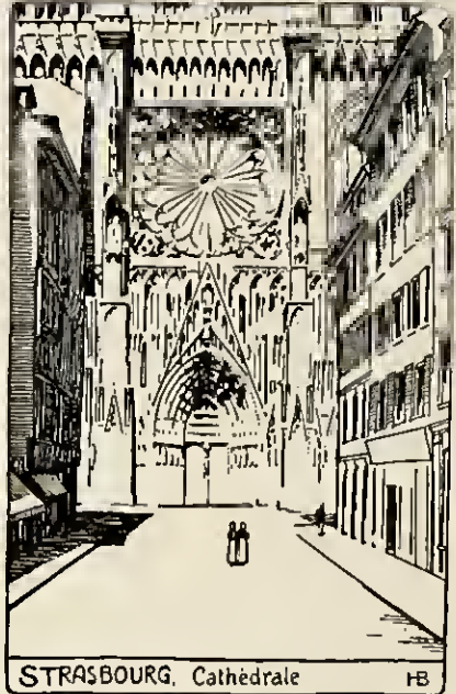
FIG. 78—STRASBOURG, CATHEDRAL The Rue Mercière leads right to the central entrance of the cathedral. The effect is good because the street is narrow and short (see plan Fig. 354) and the houses lining it are not too high. The appearance of the highly symmetrical central features of the western facade can thus dominate the view. If the street were longer and wider the unsymmetrical tower development and perspective diminution would become disturbing factors.
